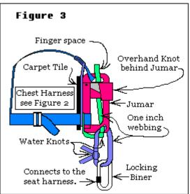
With your now free right hand grab the webbing ends and put them through the eye from the bottom side to the top. Pull tight to make the knot.
