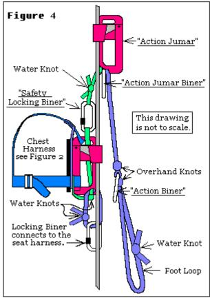
webbing through the bottom hole of the "action Jumar" and through the "safety locking biner" that is clipped onto the loop at the top of the chest harness Jumar. Be sure that the "safety locking biner" is held up tight when you tie your water knot. (See Figure 4.) I also sewed the ends down.
