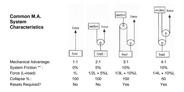
\*\* Good low friction pulleys generally are in this range, some are much worse. At lower loads, bearings are more efficient than bushing but at higher loads this can reverse. Also the force to bend kermantle rope increases with load (inner fibers sliding over each other under increasing tension). The addition of edge rollers and directional pulleys will also contribute to system friction and should be considered.
