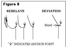
(See Figure 8.) The loosely redirection biner rebelay (deviation) can be passed by rappelling an inch or
