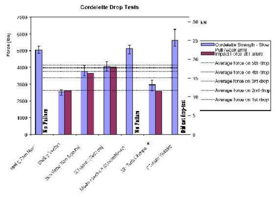
\* Ultratape was tested with a sewn eye in the pull-tests and a tied eye in the drop-tests.
