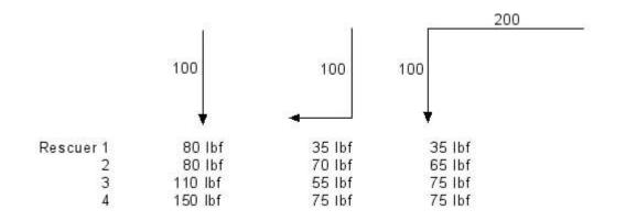
The 1<sup>st</sup> test is a vertical pull on 100 foot of rope and no change of direction.
