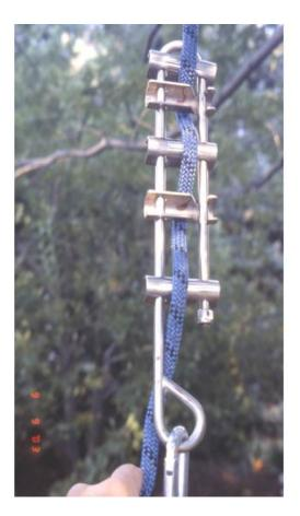
For our testing we removed the 6<sup>th</sup> bar completely from the rack, so it could not interfere in any way with the test. We would release the test mass from varying heights, which would give different lengths of rope between the belayer and the rappeller and different lengths of rope between the anchor.
