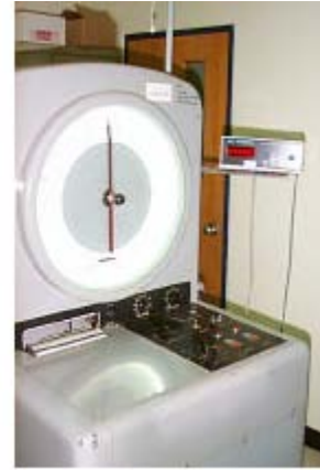
(a) The CIT tensile testing machine cross heads (b) Dial controls (The rope is to hold the pipe bollards in place when the specimen breaks)
