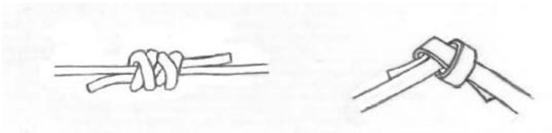
(a) Double Fisherman's Knot in rope (b) Tape Knot in tape
