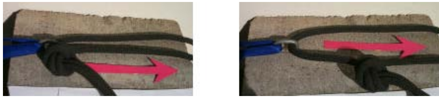
(a) The Overhand knot against the sling (b) away from the sling The arrow indicates the direction of pull. Figure 11
