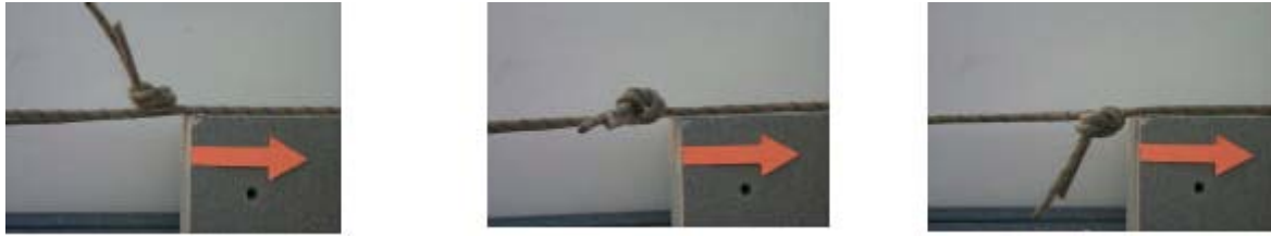
(a) Tails up (b) Tails level (c) Tails down Knot tails on the reverse edge. The arrow indicates the direction of pull. Figure 13
