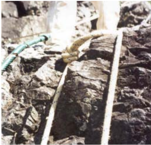
(a) The Bungonia cliff detailing the knot going over the 25° edge Figure 6 (b) Profile of the Bungonia cliff edge.
