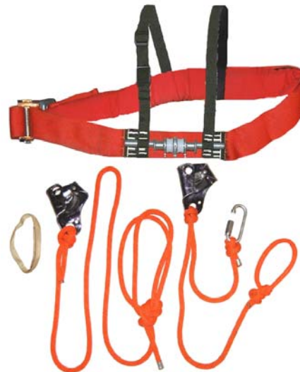
Fig 3b: This Mitchell has been reduced to minimum weight (1200 g) and bulk without reducing climbing efficiency. It uses 8 mm rope instead of sewn foot loops, a Flash Bar roller box and two Petzl Basics. The tan webbing (left) is the "chicken loop" loop for the upper ascender. The other ascender uses a sit-harness tether instead of a chicken loop.
