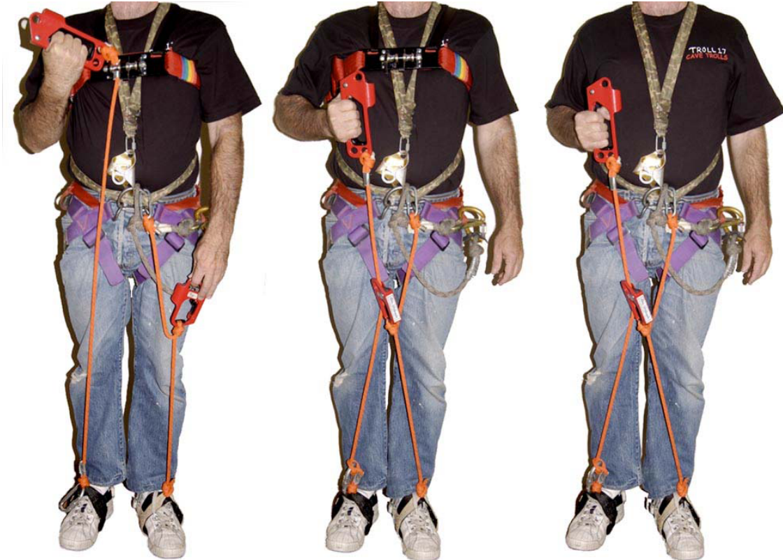
Fig 2: The standard Mitchell System with Croll addition is shown at left. The Croll does not interfere with normal Mitchell System ascents. To convert to a Frog, first attach the Croll to the main rope. The long foot line is then shortened by twisting it into a carabiner, then the lower ascender is clipped into the foot loop line and adjusted to proper height (center photo). The roller box is disconnected from the main rope entirely. The long cowtail is used as the Frog safety tether. For short drops or sequential pitches, the chest box is not used and the Frog System is used exclusively (right photo). There are several possible variations to the conversion shown here depending upon the initial Mitchell configuration. (See figures 3 and 4)
