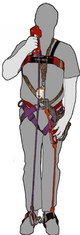
Fig 1: Wearing the Mitchell roller box over the Croll allows rapid conversion to the Frog System. The Croll serves as the Mitchell QAS.
