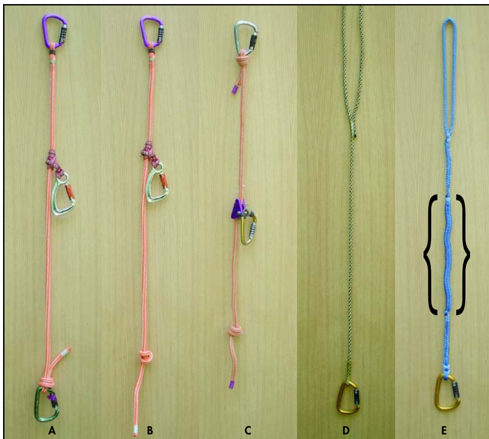
Figure 1. Five different types of tether setups, each of which uses a single length of line or cord. Because these tethers use only a single piece of line rather than a doubled line, the line must have a minimum tensile strength of 5,400 pounds.
