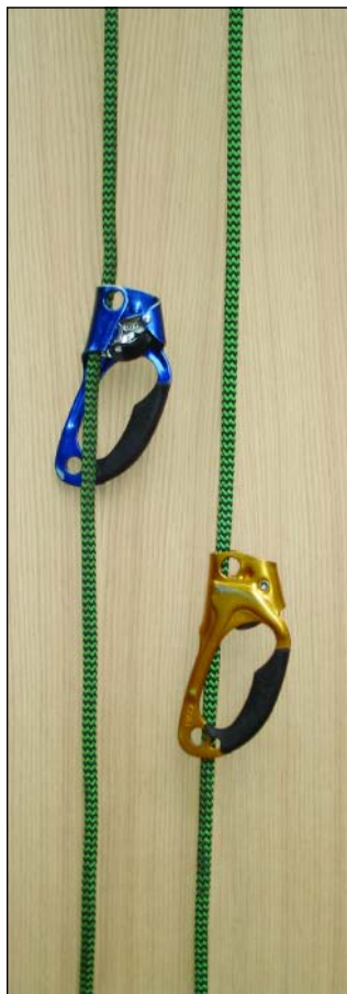
Figure 2. The left and right Petzl Ascension single-handed ascenders on the two legs of a doubled line.
