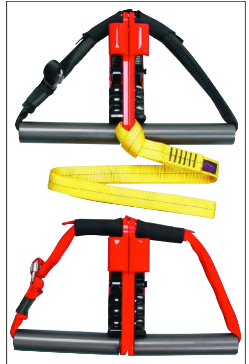
Figure 4. Mar-Bars use two single-handed CMI Ultracenders to form a single, double-handled upper ascender (with yellow strap) for the hands and two more Ultracenders to form a single lower ascender for the feet. The climber is attached to the upper ascender only and uses the lower ascender simply to assist in his or her inch-worm progression to the top. Because the climber is attached only to the upper Mar-Bar, it is recommended that another system be used as a backup.
