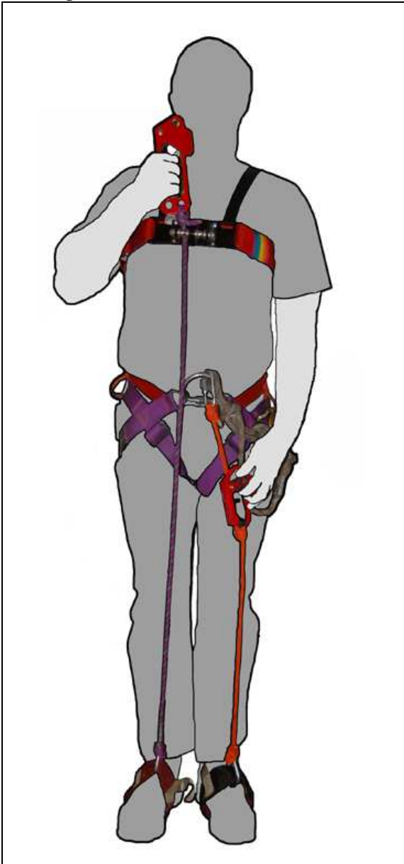
Fig. 1 The Mitchell ascending system, right handed setup. Sewn foot loops are shown, but rope loops may be used. This illustration shows the safety tether attached to the lower ascender, but either ascender may be used. Cowtails are not essential to ascending, but are included as essential vertical caving gear.
