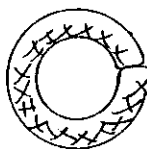
Figure #5. Three foot number five steel reinforcing rod with welded eye makes a good mud piton.
