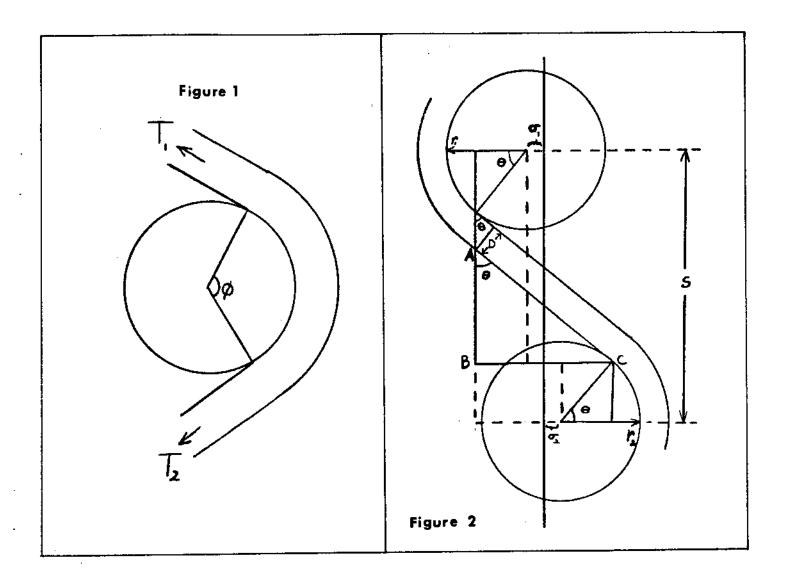
Table 1 shows a sample hand calculation of bar loadings. Since the heating of each bar is essentially proportional to the tension difference at the bar, the power into each bar need not be calculated numerically. In the sample calculation,  $\mathcal N$  was chosen as 0.25 (typical). As a further convenience in hand calculation,  $\theta$  was set equal to 1 radian for all bars (therefore  $\emptyset = 1$  or 2 rad, depending on the bar). A 200 lb. caver weight was chosen.
