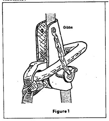
Take hold of the two ends of the 5mm rope and tie a double figure of eight knot in it close to the cam eye. Pass one end of the 5mm rope through the carabiner in your sit-harness and join the two ends. The correct length for this loop will be found by ensuring that when the Shunt is locked onto the rope under load, there is 30-50mm between the shunt and the top of your descending device. The chest activating link is then attached. Pass a carabiner through the loop at the eye of the
