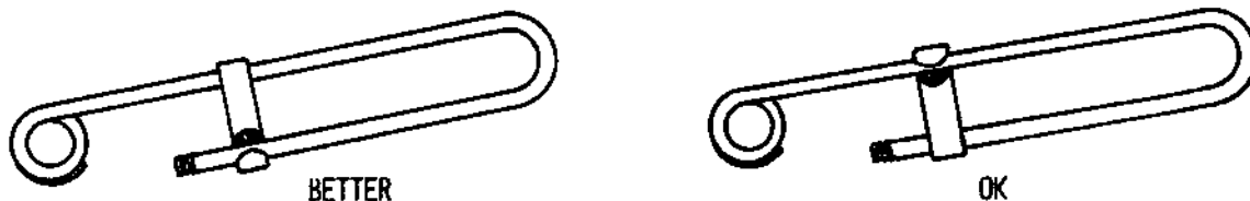
FIGURE 5. ALTERNATIVES FOR THREADING A BAR ONTO THE RACK FRAME--WITH EYE ON LONG OR SHORT LEG.
